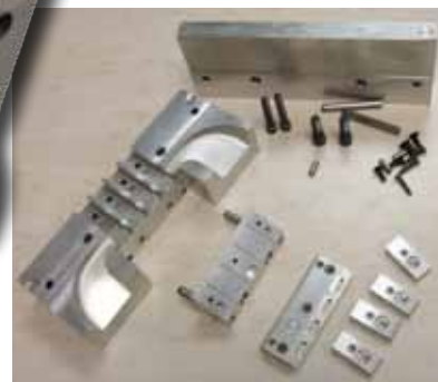
TOP RIGHT & ABOVE: Mould components, including some 3-D machining, made by Schuller Machine.
